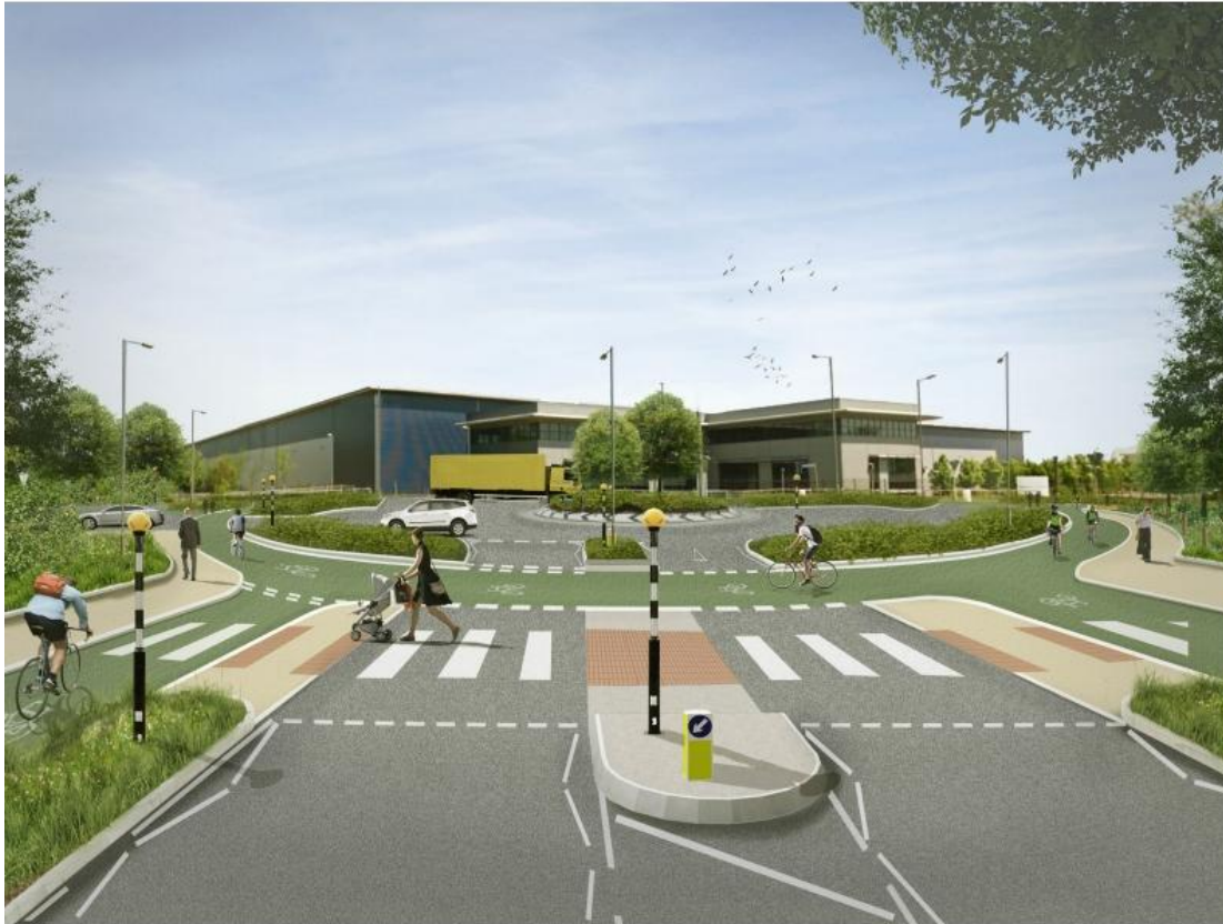
Proposed Dutch style cycle and pedestrian friendly roundabout for Boundary Way Hemel Hempstead
